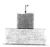
Problem Statement: 60 nm x 60 mm oak post on pine block. Given the allowable stressed, find the maximum P possible. What is the maximum P if a bearing plate is used?
